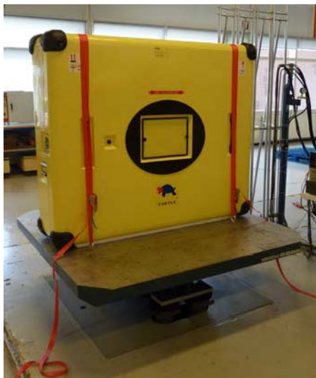
Fig. 5 – Vibration test set up
